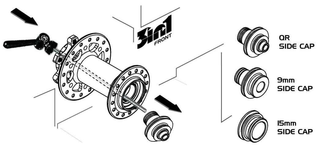
HUB MODEL: XD711SB FOR WHEELS: DRAGON FLOW TRAIL TX 29ER 1. USE QR TO PUSH THE SIDE CAP OUT OF HUB SHEEL.
