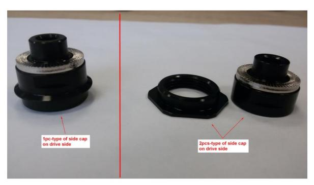
b. If it is for 12x142mm through axle (X12), please check which type of side cap is there on the drive side (cassette body side). It can be either side cap with simple cylindrical shape or a side cap also with cylindrical shape, but with small flange/skirt on it, like picture below shows:
